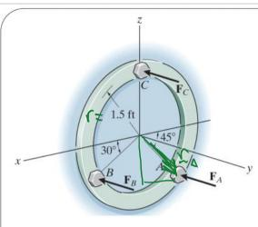
The three parallel bolting forces act on the circular plate, such that  $F_A = F_B = F_C = F > 0$ . Replace the force system by a resultant force  $F_R$  and a resultant moment  $(M_R)_o$  about the origin.
